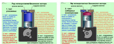
Figure 1. Principle of working of a four-stroke engine - first and second stroke
