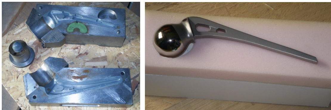
Figure 1. Tool for meltable implant model (left) and finished hip implant metal cast piece (right) (Courtesy of investment casting foundry – Livnica preciznih odlivaka Ada)
