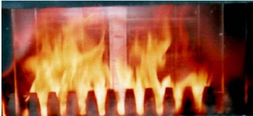
Figure 2. Combustion of fireplace bio-briquettes made of beech sawdust (weighing 433.9 g) in a fireplace manufactured by "Alfa Plam", Vranje [4]
