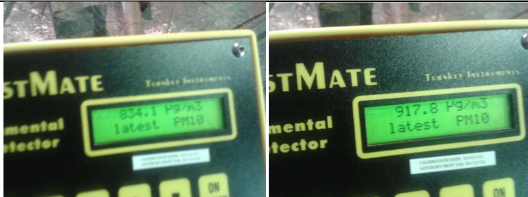
Figure 6. Measured values of the dust exiting left and right bore of tunnel T1 with filtering of air pollutants
