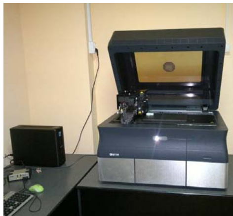
Figure 4. Objet 3D Printer Multifunctional Desktop 30 (Courtesy of Center for Numerical Simulation and Digital/Rapid Prototyping, University "Eftimie Murgu" Resita, Romania)
