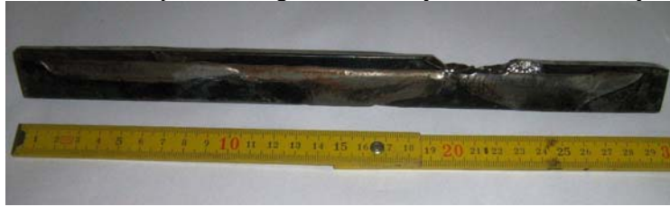
Figure 2. Damaged extraction cage knife – made by cladding
