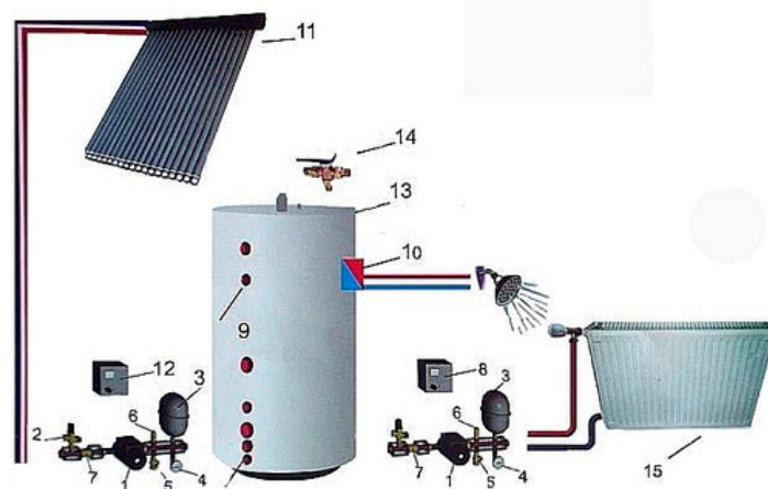
Figure 1. The use of solar collectors for heating and hot water
