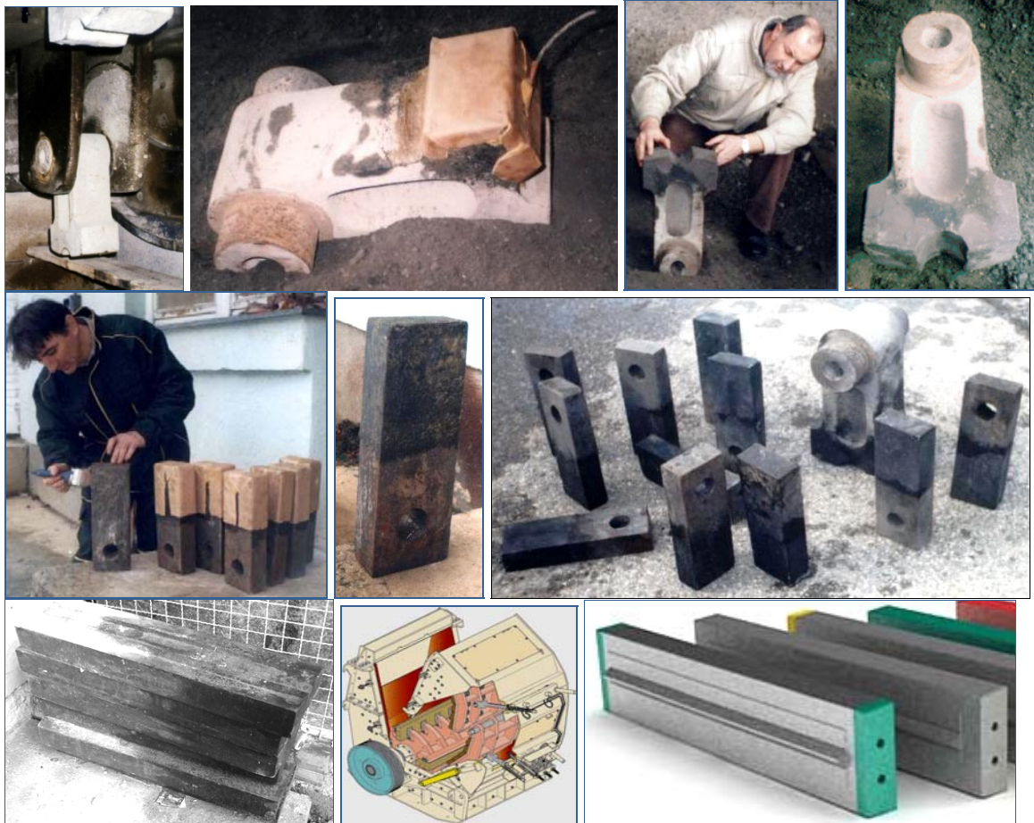
Figure 6. Hardening of the hammer for limestone crushers
