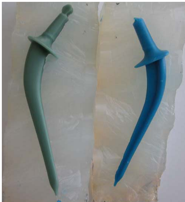
Figure 14. Models of lost wax and silicon rubber mould [5]
