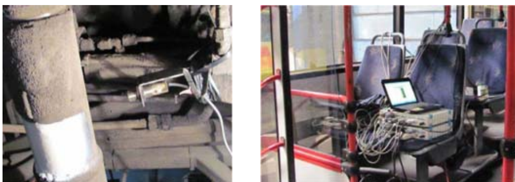
Figure 4. (a) Optical sensor for measuring speed; (b) the data acquisition device Spider 8
