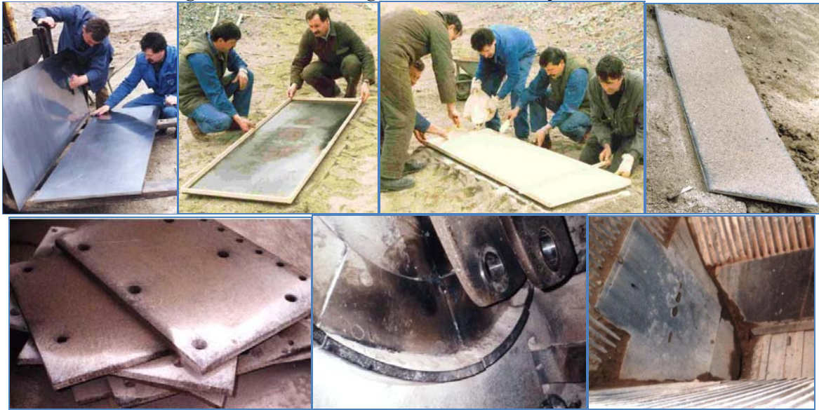
Figure 3. Production of bimetal (Č0563 + Č3160) for lining of loading baskets
