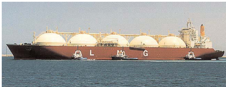
Figure 2. Tanker ship for carrying LNG from bunker-to bunker (on the left) and cross section of typical LNG chamber on the tanker designed by Moss maritime (on the right).
