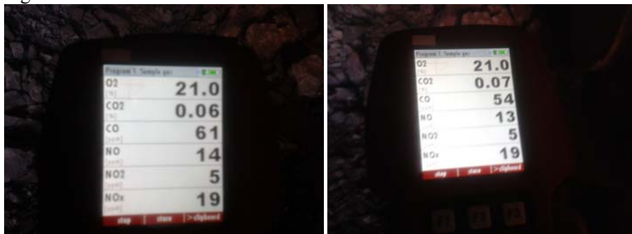
Figure 3. Measurements of gases after the explosion at the face of a) tunnel T1 – left bore b) tunnel T1 – right bore
