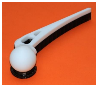
Figure 17. Hip implant ABS model with support structure
