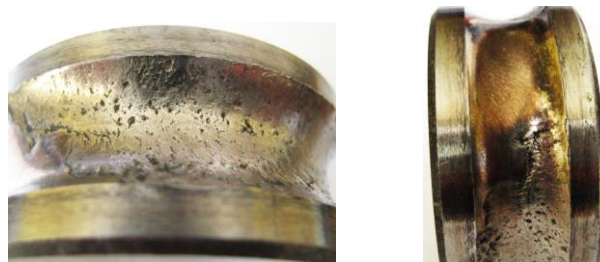
Figure 3. Fatigue wear (pitting) on the outer surface of the bearing inner track
