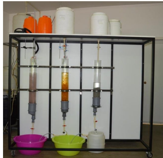
Figure 2. Pilot plant for the treatment of raw drinking water by ferrate(VI)
