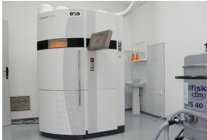
Figure 7. Formiga P100 EOS SLS machine
