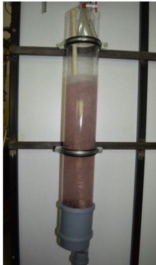
Figure 3. Reaction column for the treatment of raw water by ferrate(VI) with aeration
