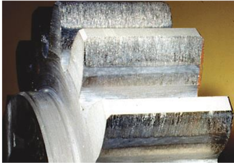
Figure 6. Gear scuffing failures [12]
