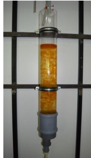
Figure 4. The reaction column for coagulation
