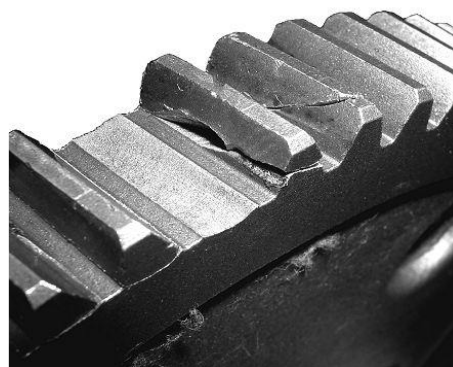
Figure 9. Breakage of more gear teeth [15]
