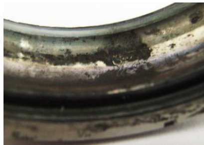
Figure 5. Fretting corrosion on the outside rolling track of ball bearing [11]
