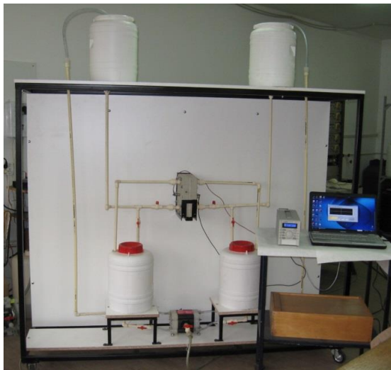
Figure 1. Pilot plant for the electrochemical synthesis of ferrate(VI)
