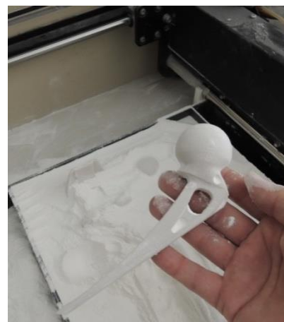
Figure 13. Printing process of the hip implants by 3DP technology
