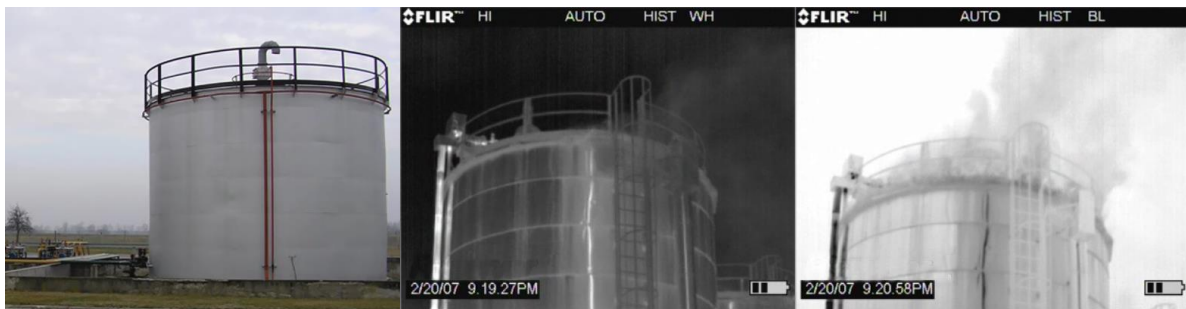
Figure 5. Detection of leakage of natural gas from reservoir, source [10]
