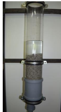
Figure 6. Filtration column with filtration sand of different granulate
