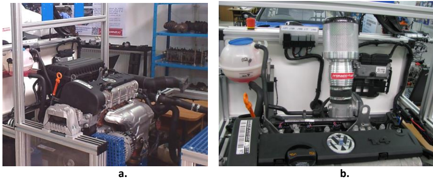
Figure 5. a – Engine equipped with original filter, b - Engine equipped with YXV filter
