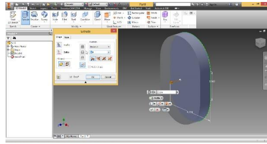
Figure 5. Creation of 3D solid model with command extrude
