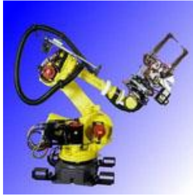
Figure 8. The Spot Welding Robots
