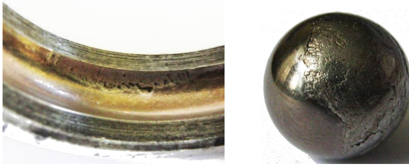
Figure 4. Pitting on the outside rolling track ball bearing and the ball
